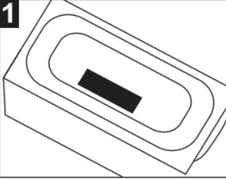
When removing tub from carton do not remove pad from tub bottom, removal voids warranty. Pads and blankets should be used to prevent damage. **DO NOT STAND** on the top of the tub.
