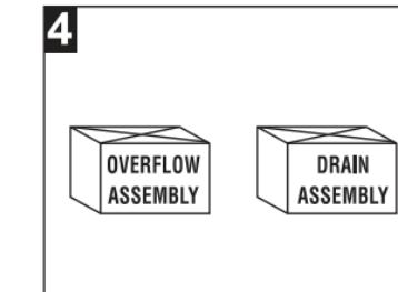
Install drain & overflow assemblies as directed by the manufacturer. **DO NOT over tighten the fittings connected to the tub. OVER TIGHTENING THE DRAIN CAN DAMAGE THE TUB AND VOID THE WARRANTY.**
