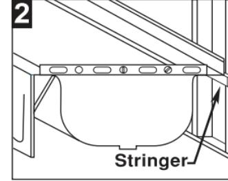
Tack the 2" x 4" stringer at a height that allows the tub to sit level, resting on the foam support pad. The stringer must run the full length of the tub. **INSTALLING THE TUB WITHOUT A FULL LENGTH SUPPORT STRINGER WILL VOID THE WARRANTY.**
