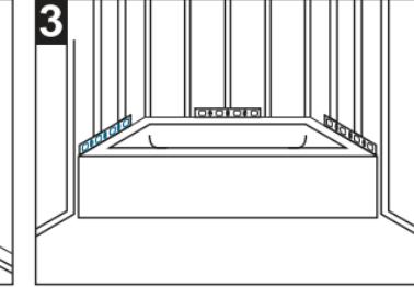
Check level in all directions. Use wood shimming if necessary. **DO NOT shim under styrofoam support pad, it is required that the foam support pad rest on the floor. The floor should be flat and level. Once tub is level permanently fasten stringer to the studs. DO NOT fasten through tub flange.**
